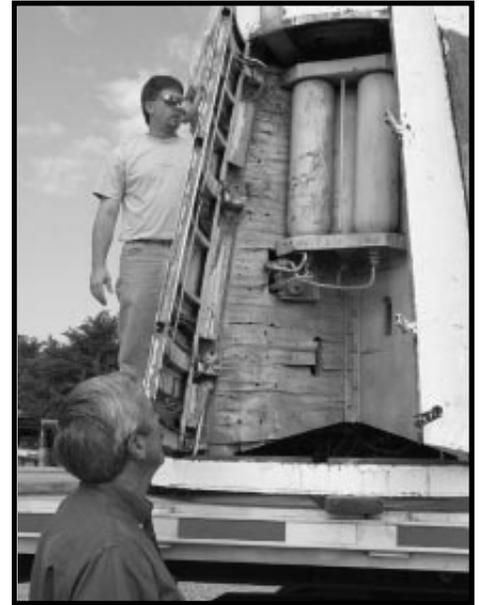
Ron Burkett, bottom, looks up into the V-2 guidance section as workers prepare the nose for shipment. All the visible components in the rocket are labelled indicating this V-2 was once on display in the horizontal position with various hatches open so visitors could see inside. The oxygen tanks visible in this photo are mounted on plywood which is beginning to rot away.
