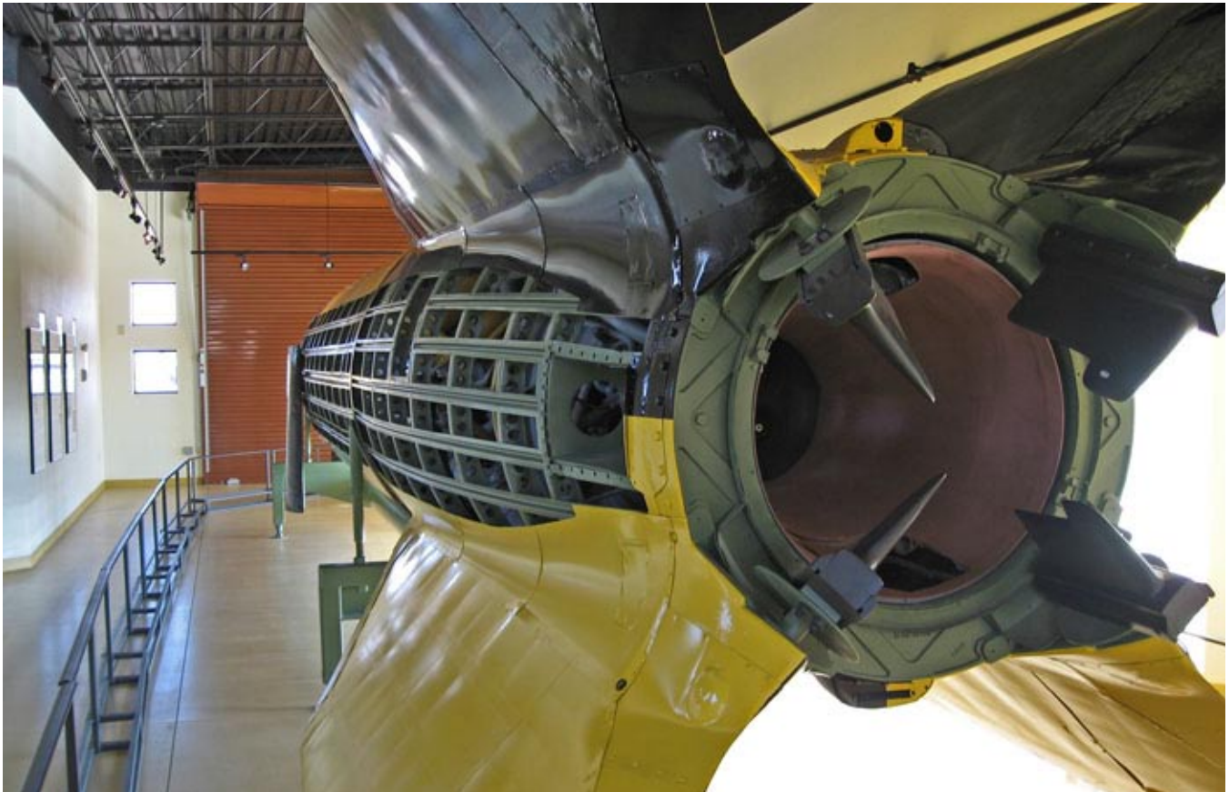
This view of the V-2 shows the cutaway side. Note the simulated carbon vanes that protrude into the exhaust area of the engine. By rotating the vanes and deflecting the exhaust one way or another, the V-2's control system kept the big rocket stable in early flight until it reached a high enough speed for the fins to work. Photo by Jim Eckles.
